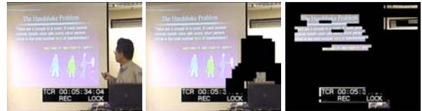
Figure 3. (left) Original image frame; (middle) segmented background; (right) detected captions for slide transition detection.
